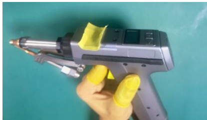
③ Use masking paper to prevent dust
